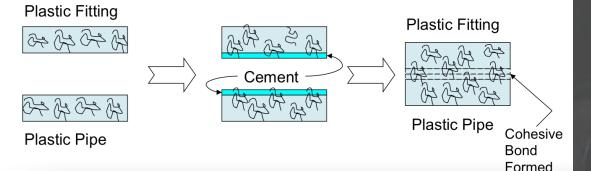
When solvent cement is applied to CPVC, the solvent softens the outer layer of material, which enables it to fuse itself with an adjoining piece at the molecular level.
