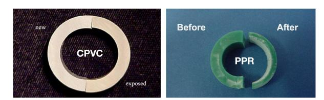
The CPVC pipe on the left was installed in the 1960's. After 23 years of installation FlowGuard CPVC did not show any signs of damage to the material or reduction of the internal diameter. The green (PPR) pipe on the right was tested in accordance with NSF P-171 (Protocol for Chlorine Resistance of Plastic Piping Materials) and showed significant signs of pipe wall erosion after only 9 and a half months.
